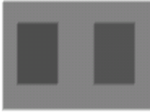
Fig. 3. Simulated contrast difference between eutectic tin-lead solder and predominantly tin based solders. Tin-lead is on the left and the other, with only 88% of the foreground-background delta gray, is on the right. Delta gray for the tin-lead “joint” is 50, which is typical for about 5 mils solder.
